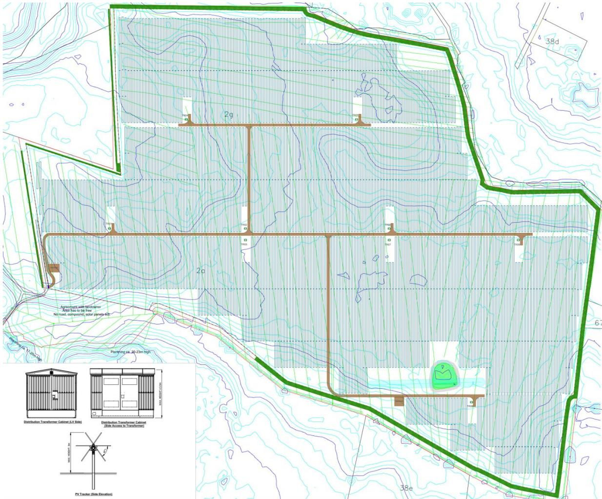
Figure 2: Provided module layout of the pv system (top view)
