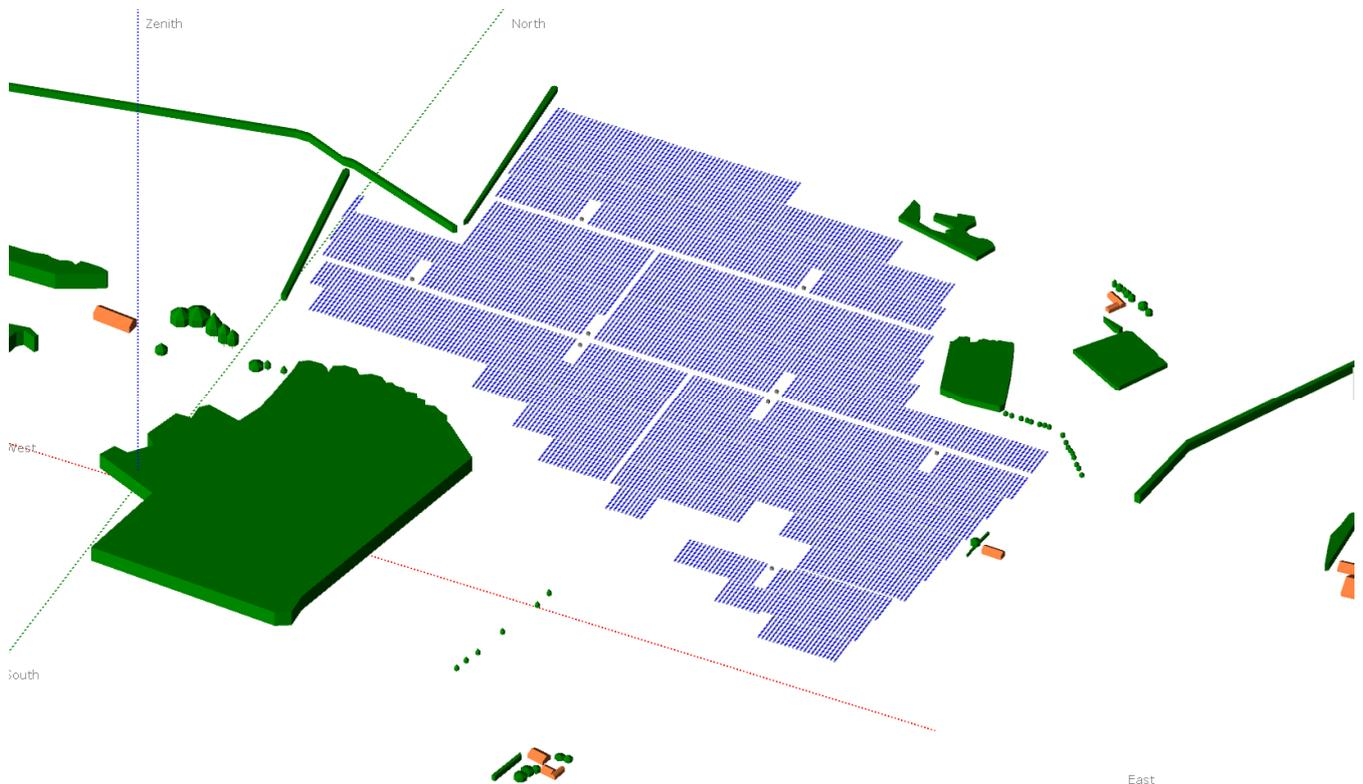
**Figure 5: Three-dimensional near shading model of the planned PV system**
